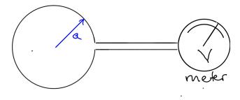
**Problem 3** (20 points) You are interested in measuring the time varying magnetic field B(x, t) at a point x. It is proposed that a planar circular loop of wire of radius a as shown in the above figure be used as a probe. We will use Farady's law to analyze how that might work.
